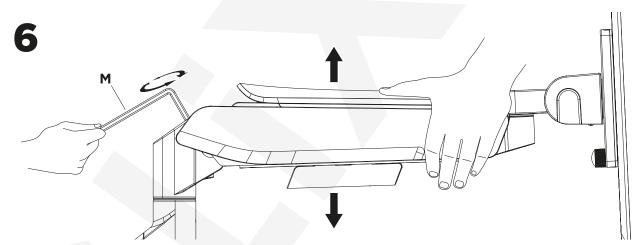
To properly balance the arm with monitor mounted, adjust the spring tension using the supplied Allen Key as follows:
