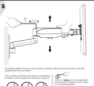
CAUTION: To avoid damage to monitors or mount, always keep the arm in a horizontal position while making adjustments. Again, ask for assistance if required.
