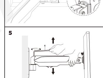
To properly balance the arm with monitors mounted, adjust the spring tension using the supplied Allen Key as follows:
