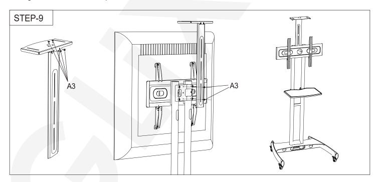
Step 9: Assemble and install the camera tray.
