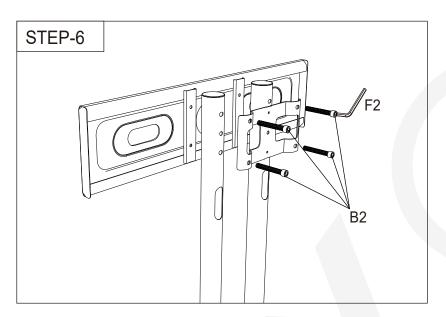
Step 6: Install the TV plate onto the tubes.
