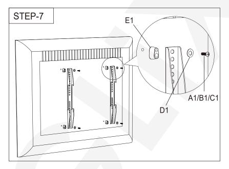
Step 7: Install the TV bracket onto the back of the TV.
