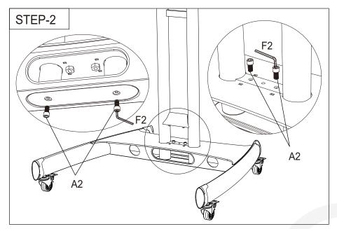
Step 2: Insert the tubes into the base and tighten the screw.
