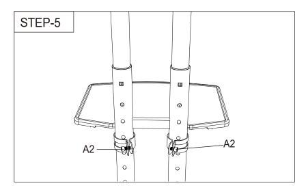
Step 5: Install the tray bracket onto the tubes.
